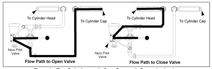
Figure 4 – Flow Path: Automatic Open Pneumatic Pump check valve
