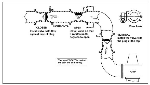
Figure 1 - Liquids with Suspended Solids
