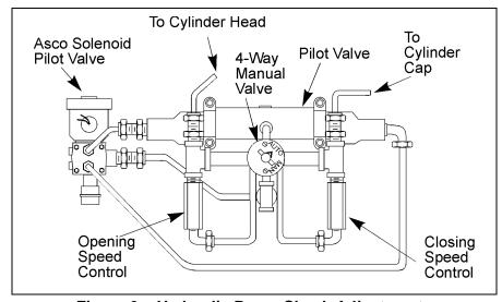
Figure 9 - Hydraulic Pump Check Adjustments
