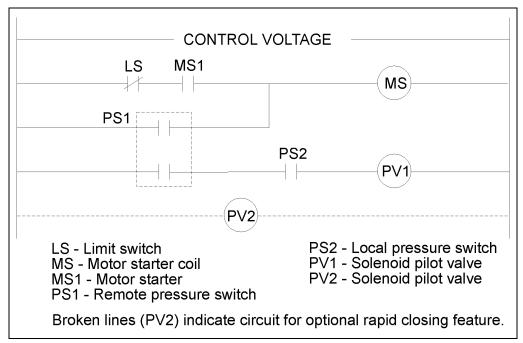
Figure 3 - Wiring Diagram
