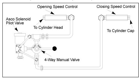
Figure 8—Pneumatic Pump Check Adjustments
