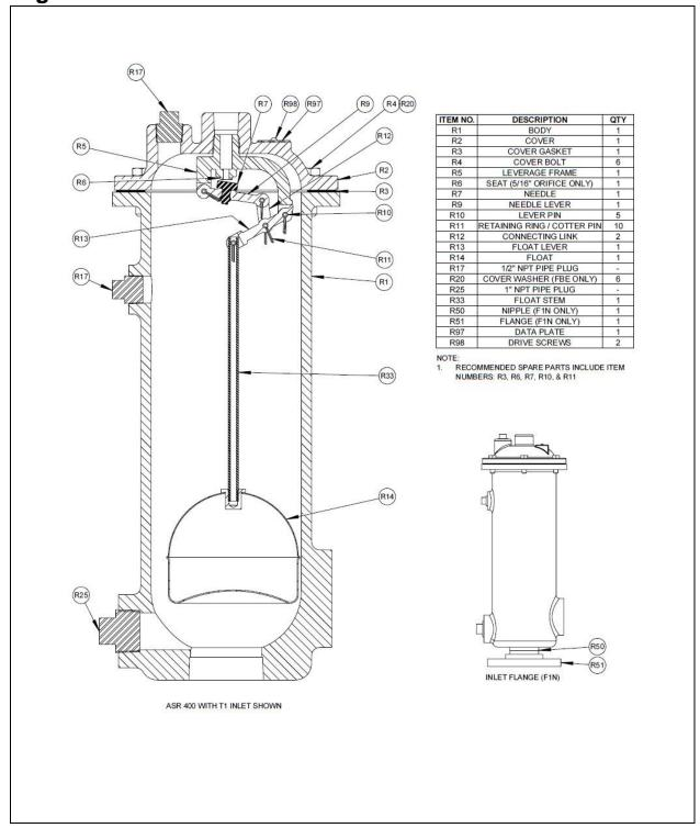
Figure 1: ASR-400 Sewage Air Release Valve
