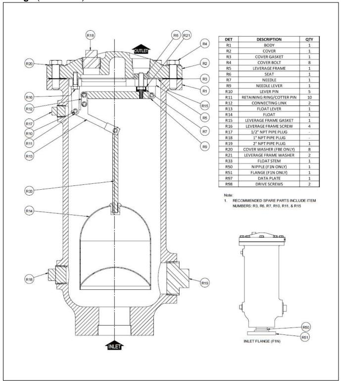
Figure 2: ASR-450 Sewage Air Release Valve
