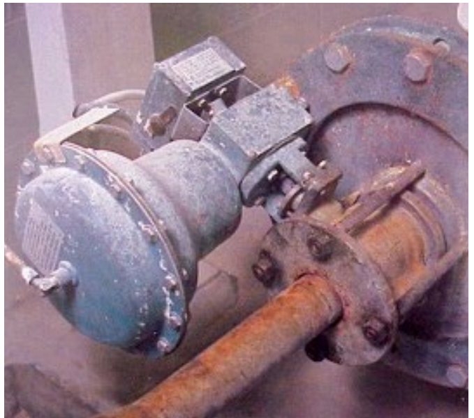
DeZURIK RCV Rotary Control Valve in abrasive kaolin clay slurry application.
