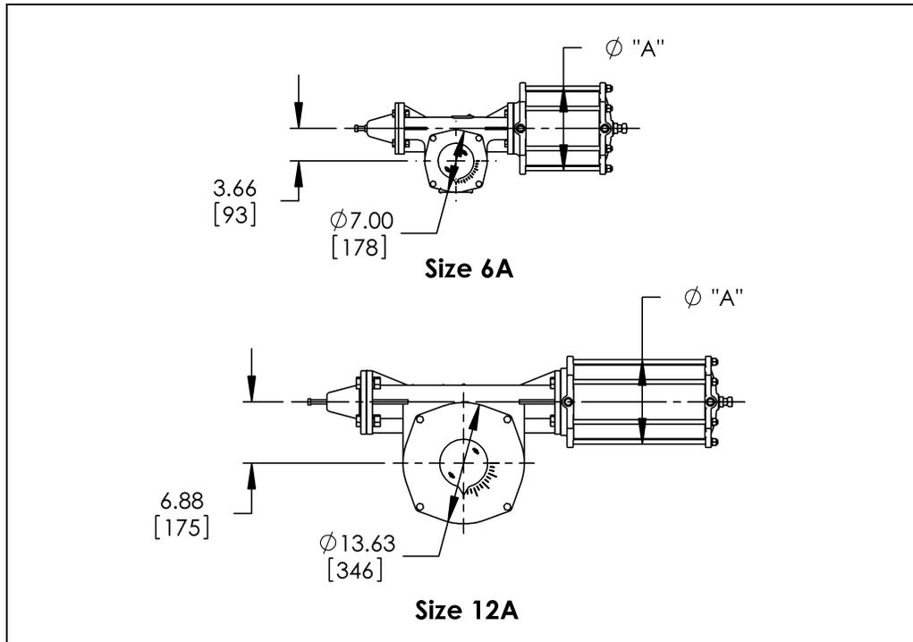
Figure 1 - Actuator Identification
