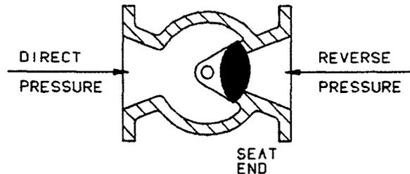
**Figure 2 – Pressure Direction**
