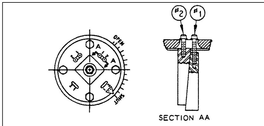
**Figure 3 – 24" thru 36" Key and Lockscrew Arrangement**
