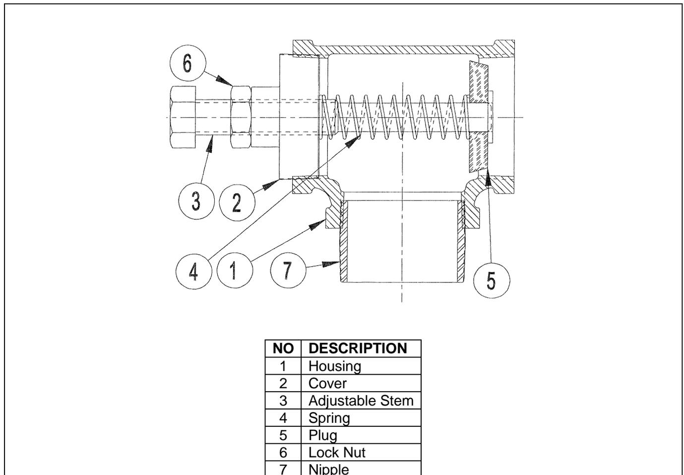
**Figure 1: DAT Double Acting Throttling Device**
