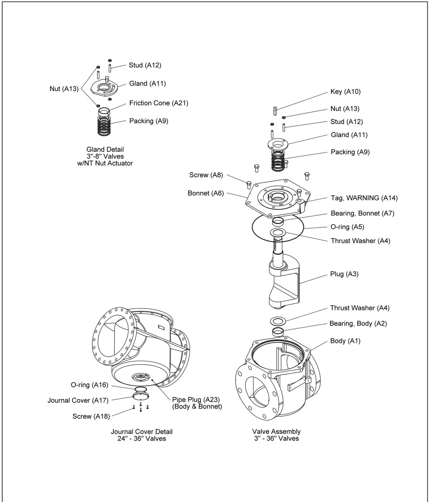
**Figure 3—Parts Identification**
