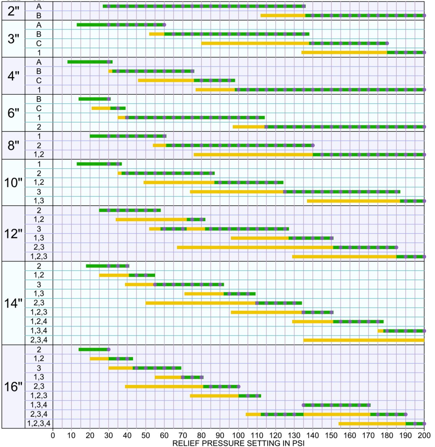
█ OPTIMAL RANGE OF RELIEF PRESSURE SETTINGS, BASED ON PERFORMANCE AND COST. NOTE THAT USING AN OVERLY-STIFF SPRING SET RESULTS A HIGHER PRESSURE RISE ABOVE THE RELIEF PRESSURE SETTING IN ORDER TO FULLY-OPEN VALVE. SPRINGS A, B, AND C ARE STAND-ALONE SPRINGS, WHILE SPRINGS 1, 2, 3, AND 4 ARE THE COMPONENTS OF A NESTING SYSTEM OF SPRINGS WHICH ARE MIXED AND MATCHED AS NEEDED THROUGHOUT THE PRODUCT LINE.
