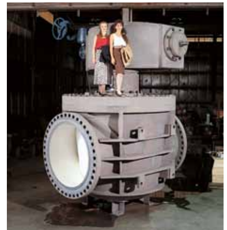
MWD of Southern California 54" (1400mm) Cone Valve Etiwanda Project
