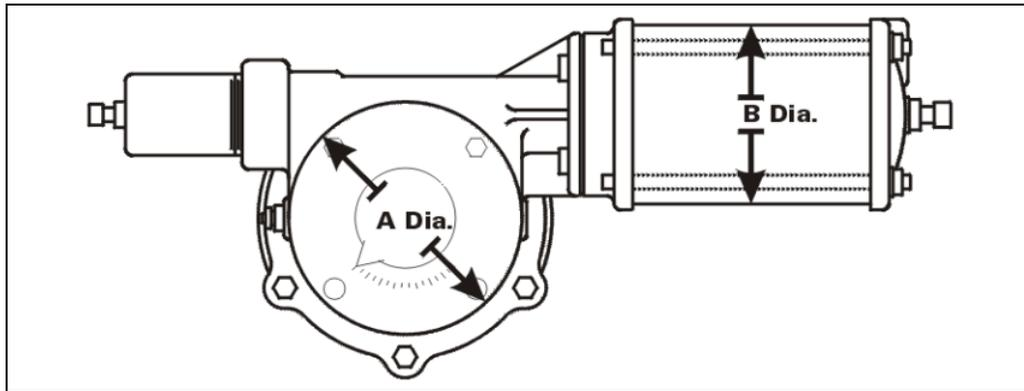
**Figure 1 - Actuator Identification**
