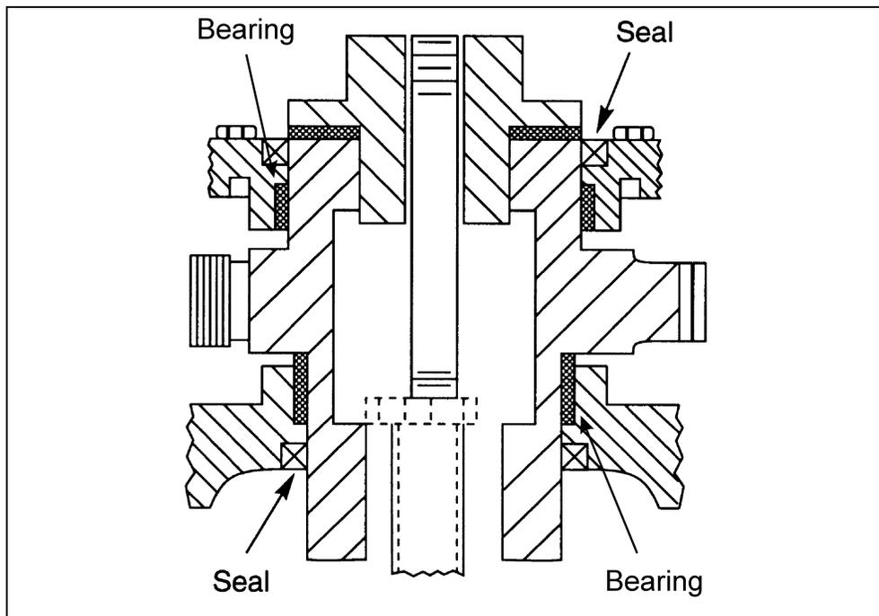
**Figure 6 – Location of Actuator Seals and Bearings**
