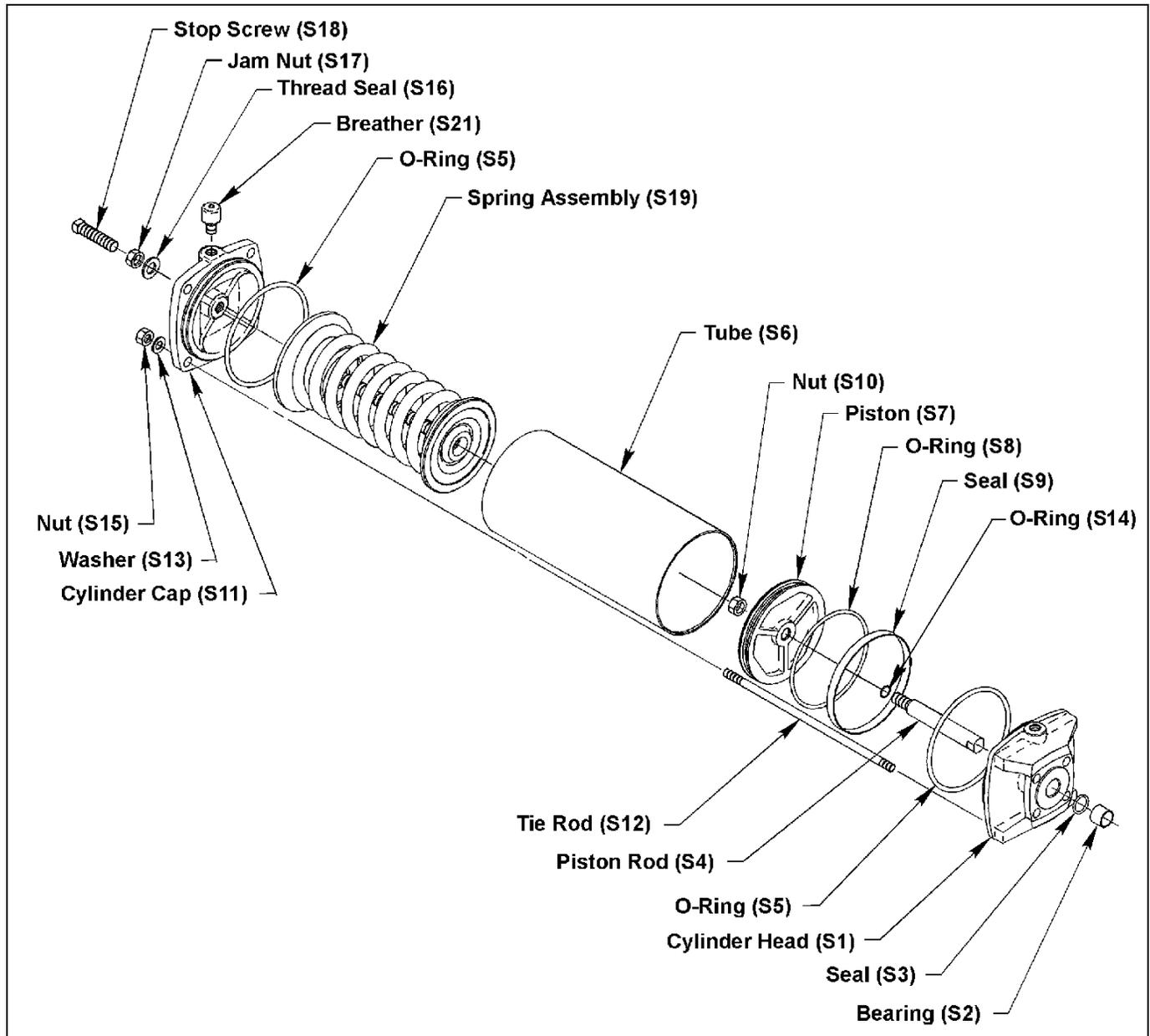
**Figure 4—Cylinder Assembly**
