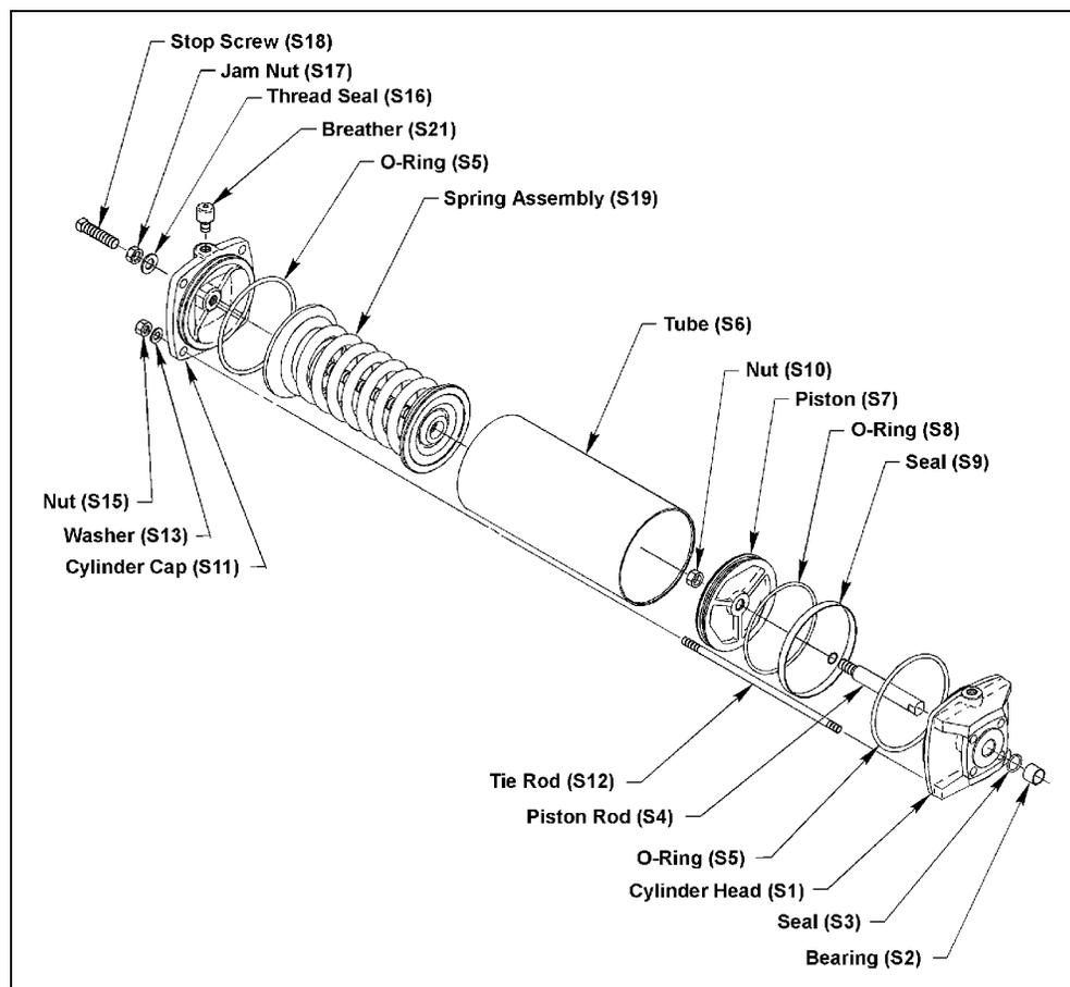
**Figure 6—Cylinder Assembly****Spring-Return Cylinder Reassembly**
