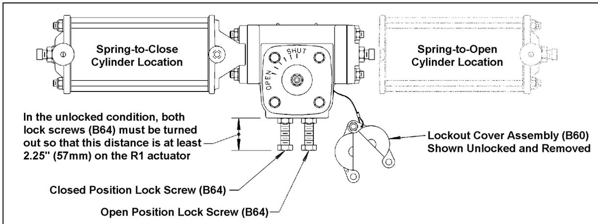
Figure 8—Unlocked Condition
