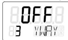
You only need to set this parameter if you want to have the total stroke in mm displayed at the end of the initialization phase. To do this, select the same value in the display to which you have set the carrier pin to the scale on the lever or the next highest position in intermediate positions.
