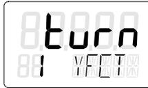
3. Switch to the second parameter by pressing the operation mode key  $\square$  briefly. This has set automatically to 90°.
