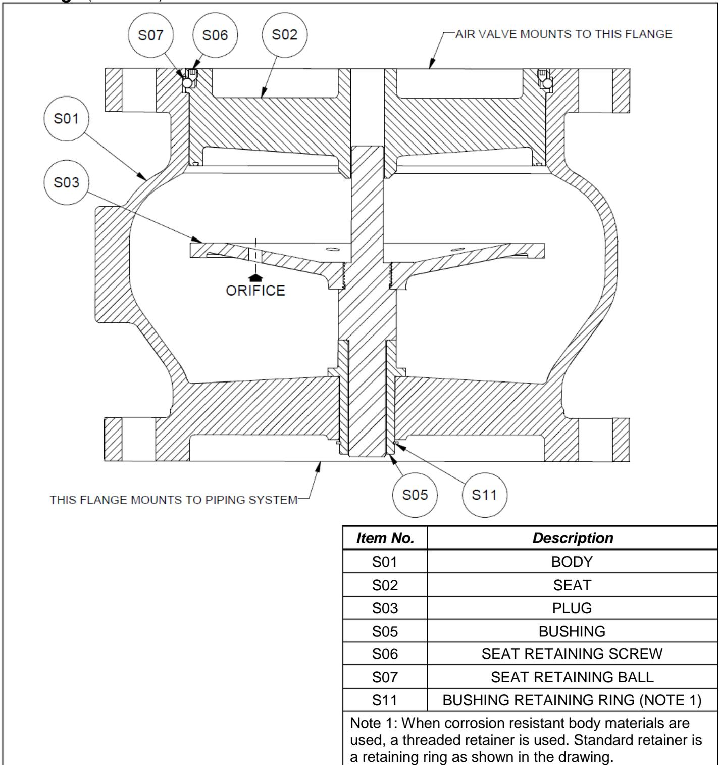
**Figure 3: CSV-1600A Surge Check Valve Sizes 3-18" (80-450mm)**
