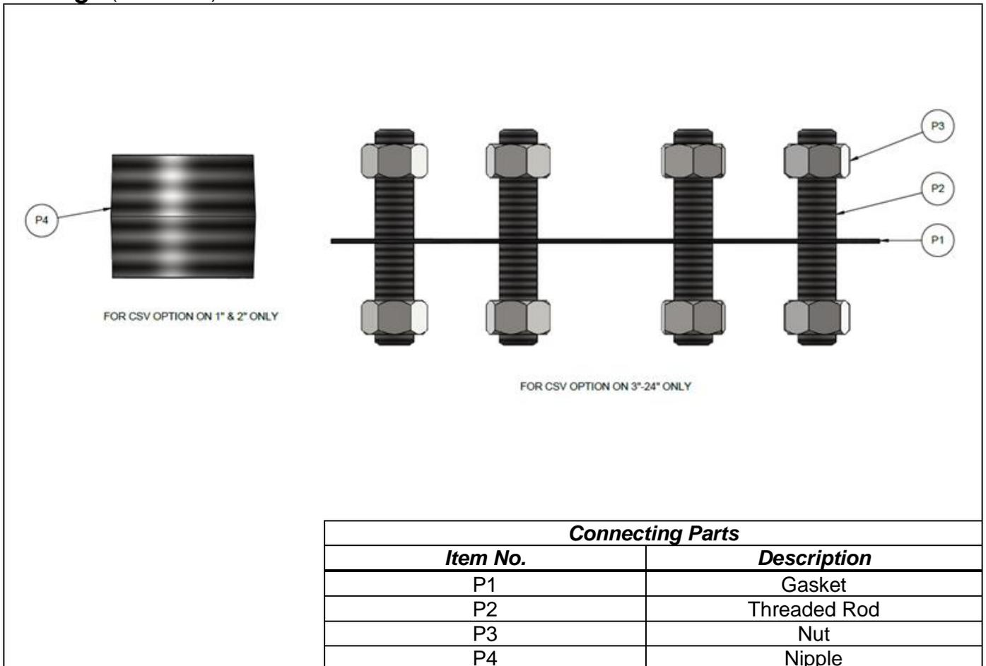
**Figure 4: Connecting Parts**
