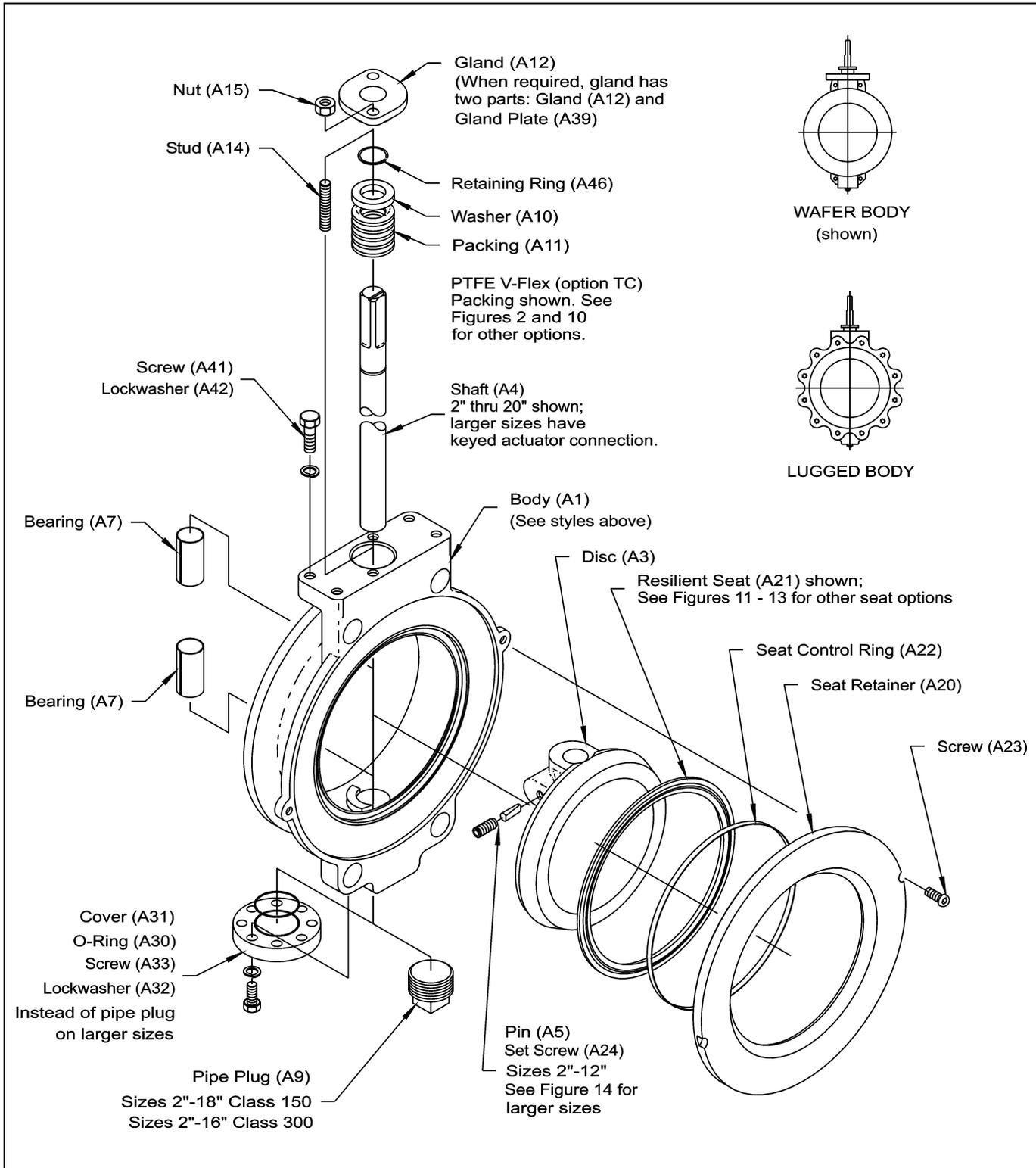
**Figure 1 – Component Identification**
