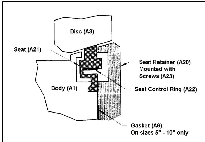
**Figure 11 — Resilient Seat Option**
