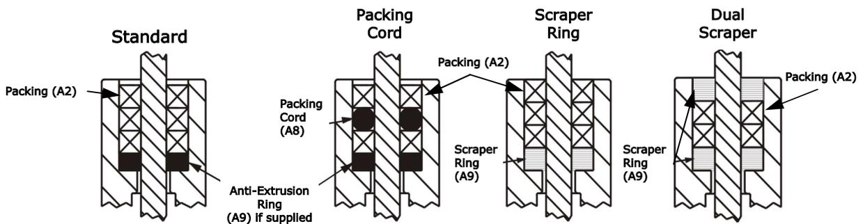
**Figure 3—Packing Detail**
