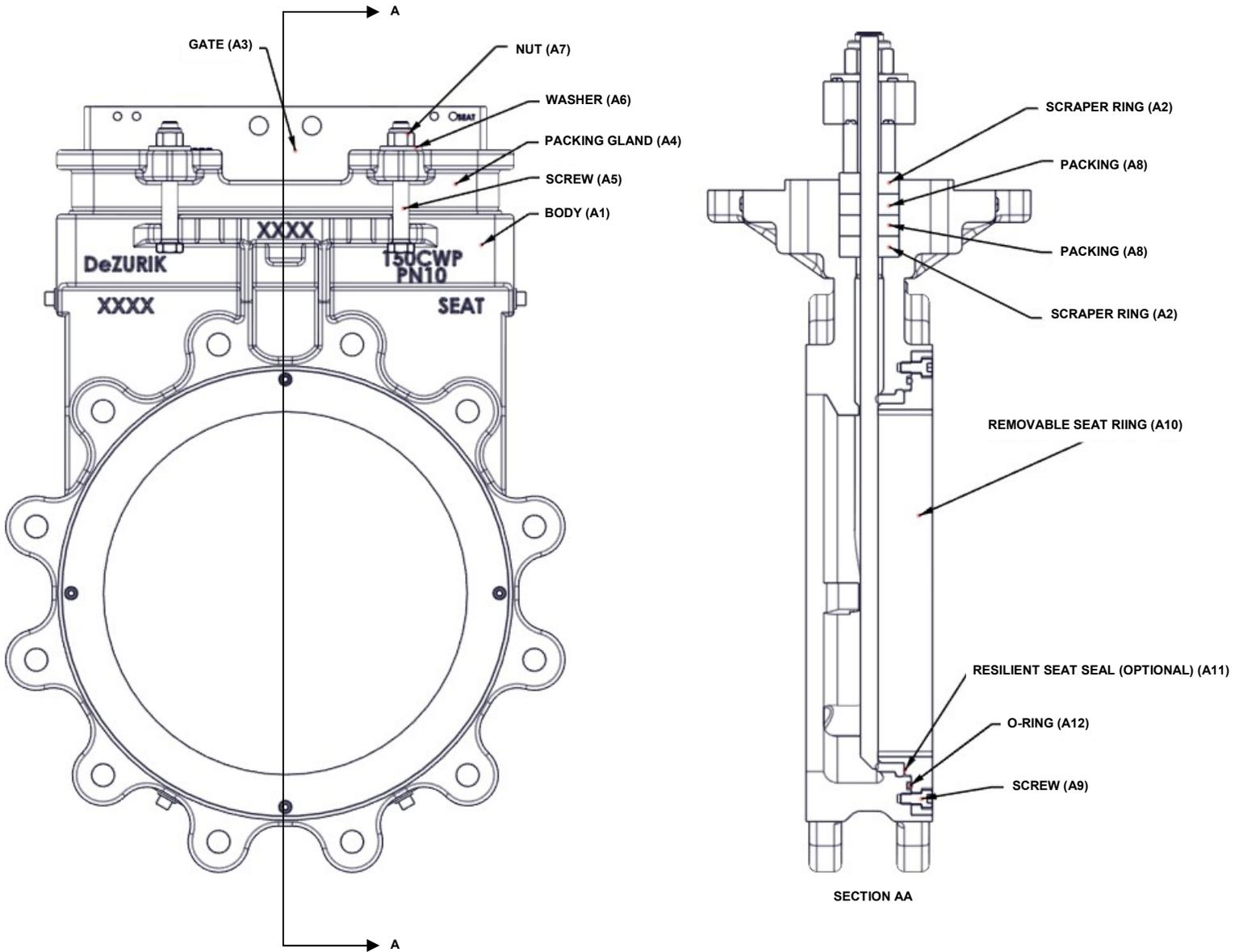
**Figure 2—Component Identification**
