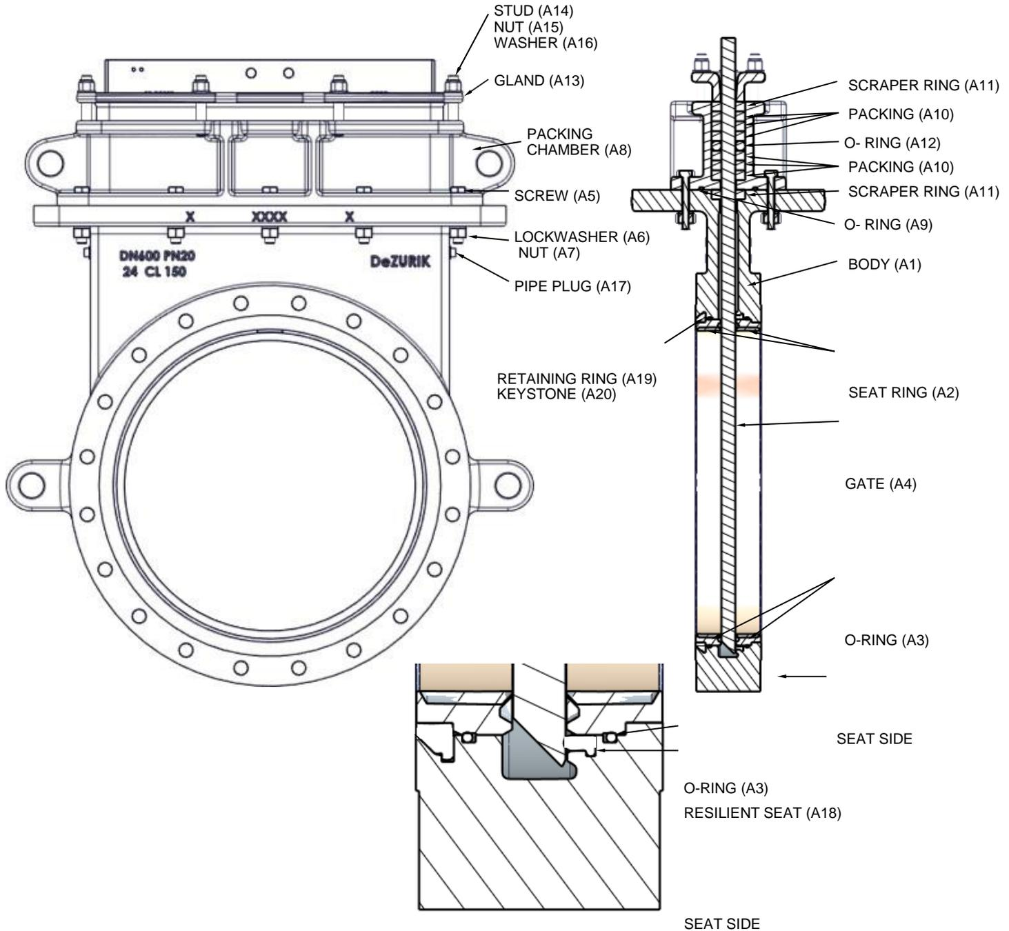
**Figure 1—Component Identification**
