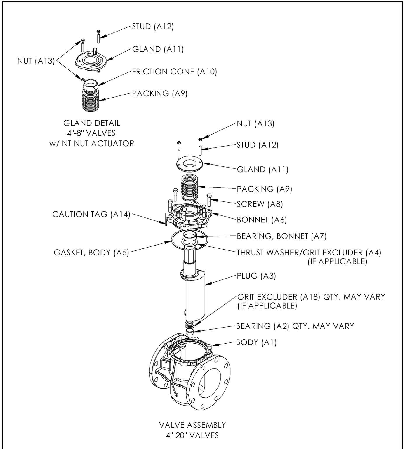
Figure 3 – Parts Identification
