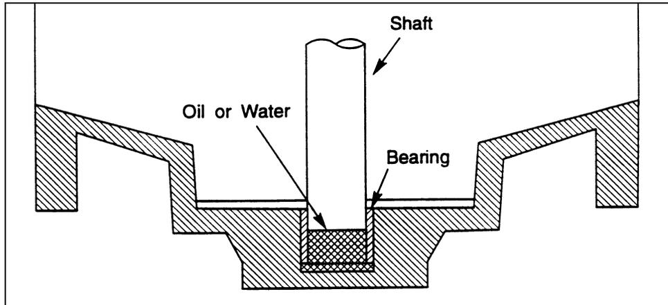
Figure 6 — Hydraulically Removing the Lower Bearing
