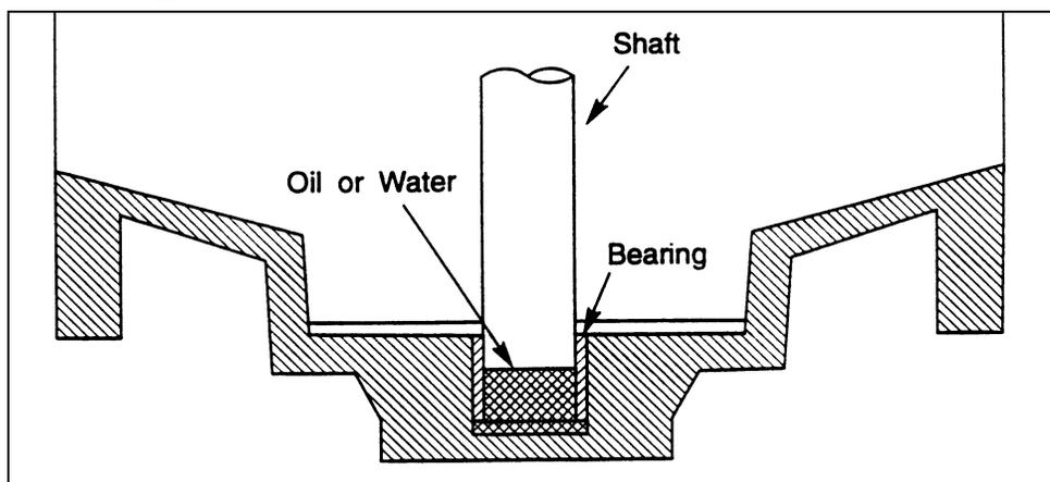
Figure 3 — Hydraulically Removing the Lower Bearing
