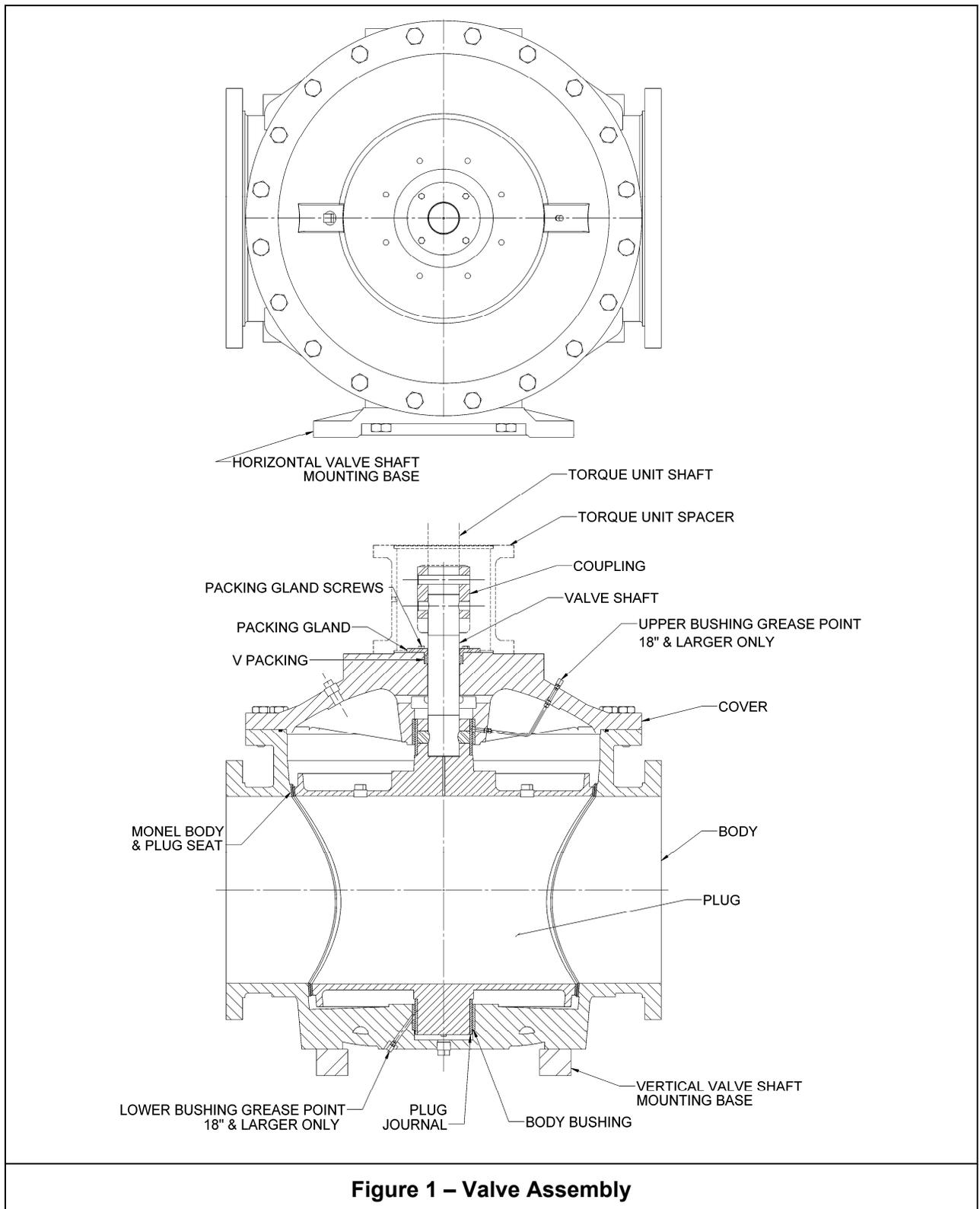
**Figure 1 – Valve Assembly**
