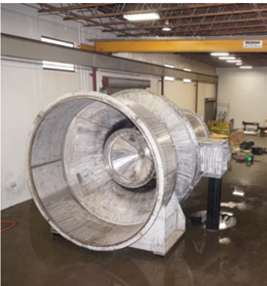
A Hilton fabricated 60" Fixed Cone Valve with installed hood, prepared to ship to a dam in the United States.
