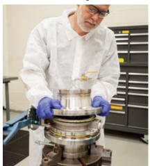
test to ensure sealing capability is maintained. The pressure test equipment is dedicated for clean valve testing only. Valves are pressure tested with nitrogen gas to ensure no moisture is introduced to the cleaned valve.
