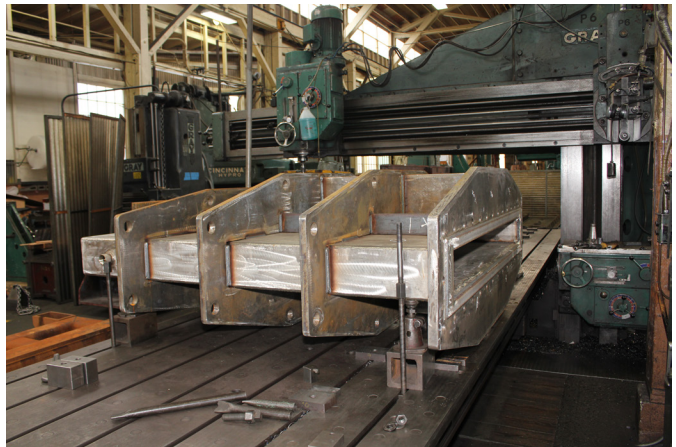
In-house machining, 72" Bonneted Knife Gate Valve
