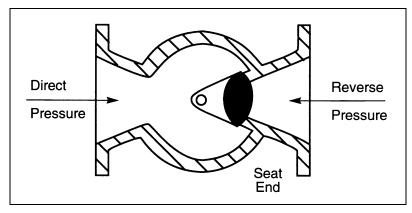
Figure 1 - Direct and Reverse Pressure Detail
