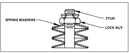
Figure 2 – Spring Washer Stackup
