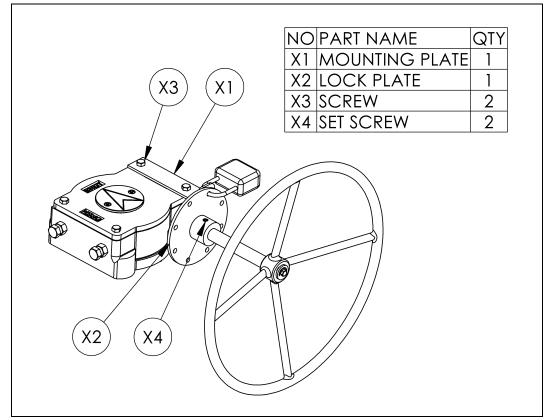
Figure 4 — Lockout Parts
