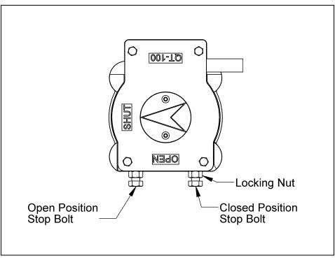
Figure 2— Locking Screws and Travel Stops
