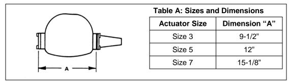
**Figure 1 - Actuator Sizes and Dimensions**
