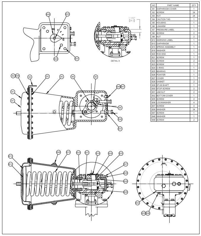
Figure 1 - Parts Identification
