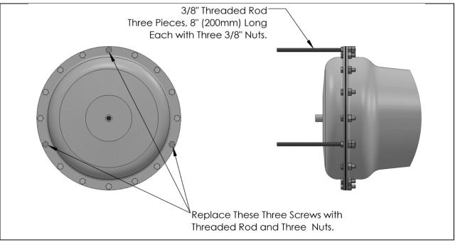
Figure 2—Stud Requirements For Diaphragm Cover Removal
