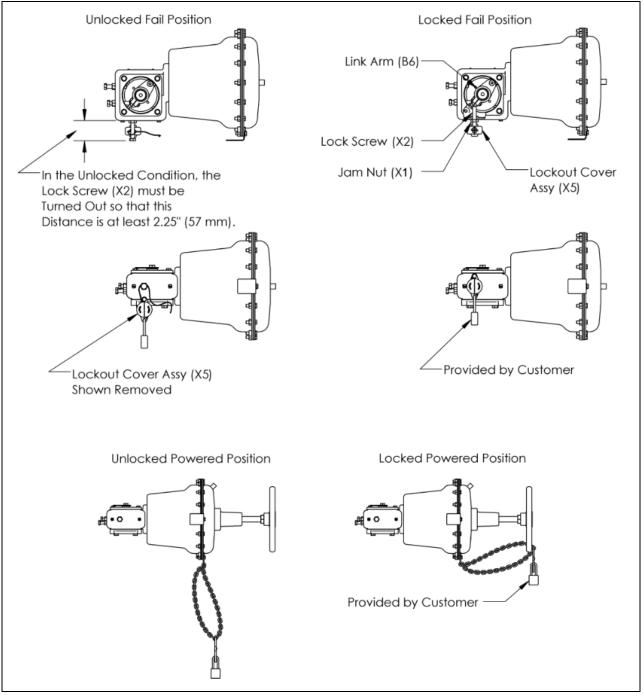
Figure 3—Lockable Model, Component Identification
