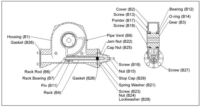
Figure 6 – Actuator Parts Identification
