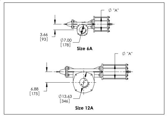
Figure 1 - Actuator Identification
