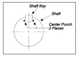
Figure 5 - Shaft Key Staking
