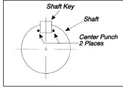
Figure 9 - Shaft Key Staking
