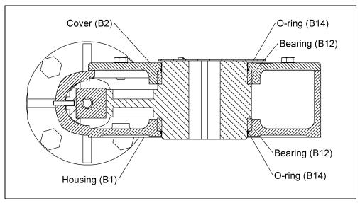
Figure 7 - Bearing and O-ring Locations
