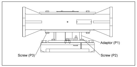
Figure 4 – Connecting Parts Identification
