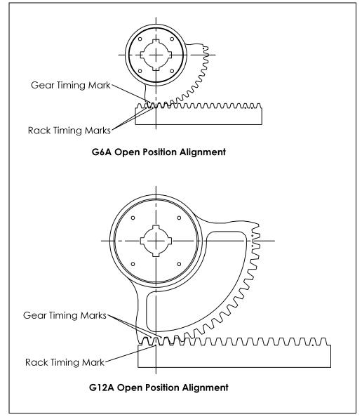
Figure 8 - Gear and Rack Alignment
