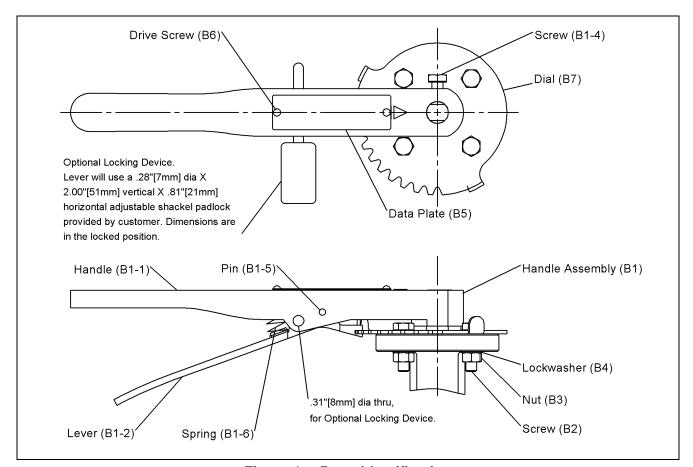
Figure 1— Parts Identification
