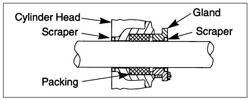
Figure 2 – Cylinder Repair Component Locations
