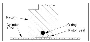
Figure 2 - Piston Seal Installation
