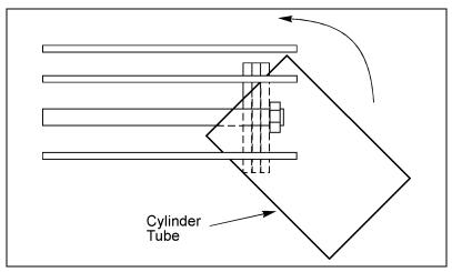
Figure 3 – Installing Cylinder Tube
