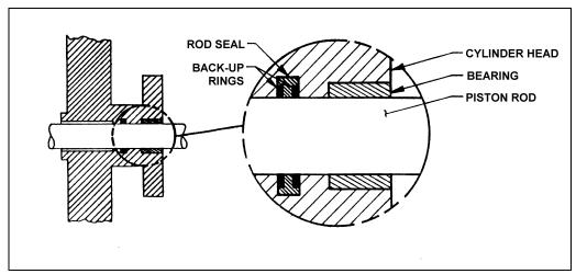
Figure 1 – Cylinder Component Identification
