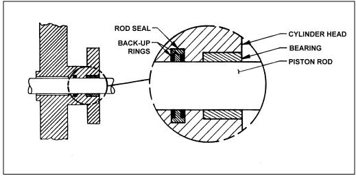
Figure 1 – Cylinder Component Identification
