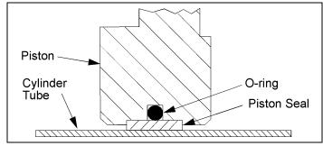
Figure 2 – Piston Seal Installation
