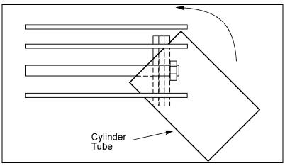
Figure 3 - Installing Cylinder Tube
