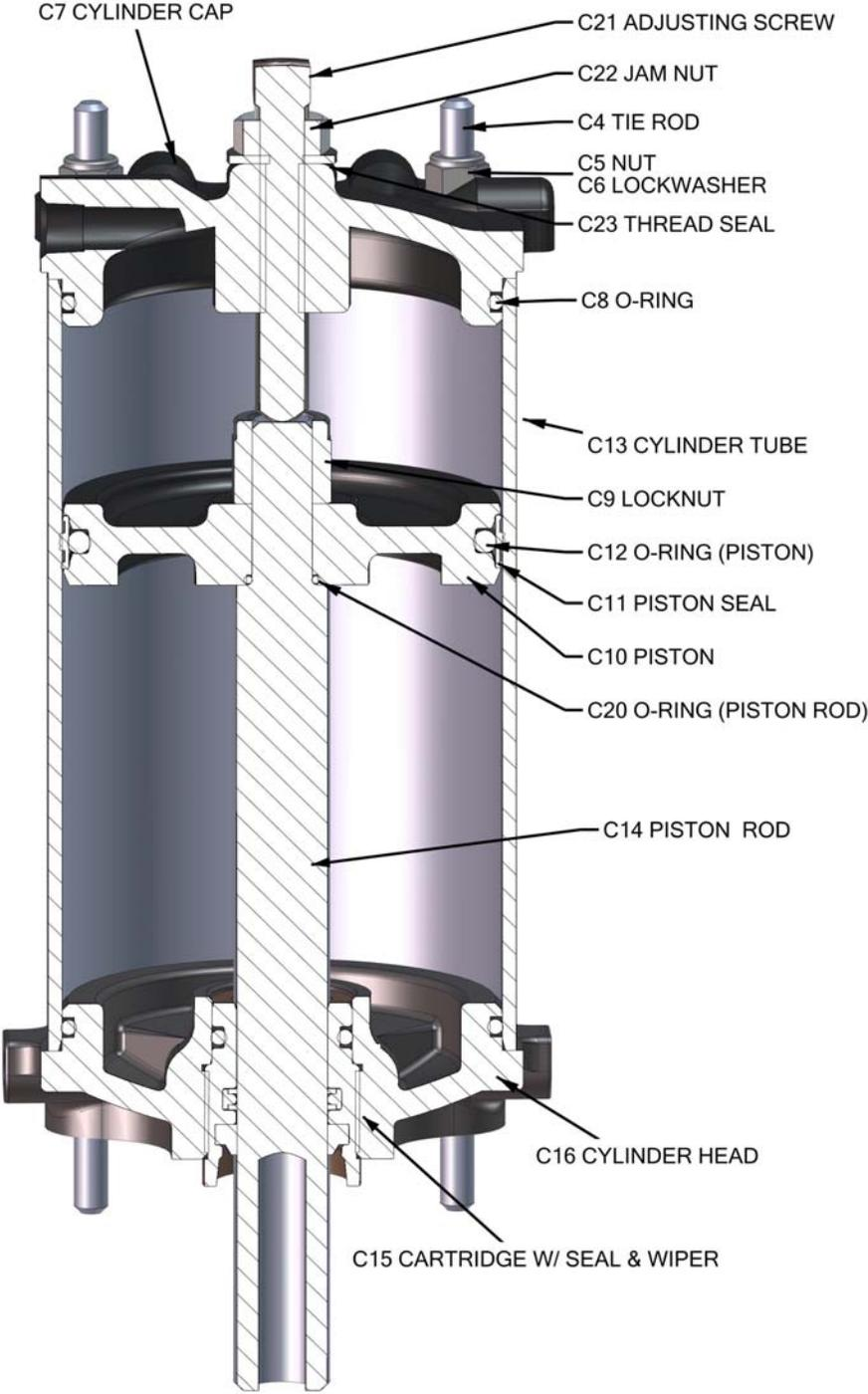
Figure 2: Component Identification
