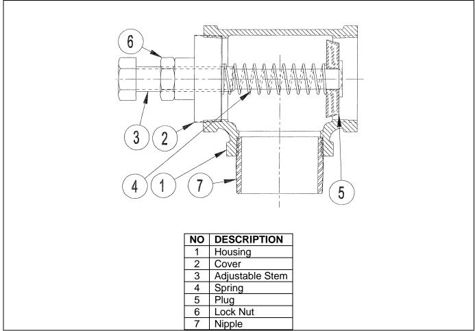
Figure 1: DAT Double Acting Throttling Device
