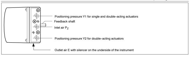
Fig. 6 Pneumatic connection
