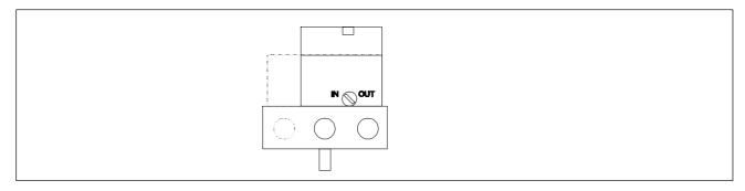
Fig. 7 Purging air changeover switch above the pneumatic terminal block, view of the device on the pneumatic connection side with the cover open
