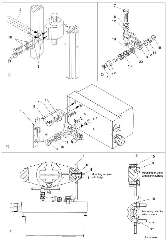
Fig. 3 Assembly sequence (linear actuator)
