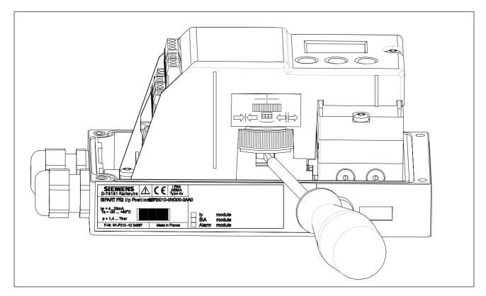
Fig. 2 Fixing device for the slip clutch
