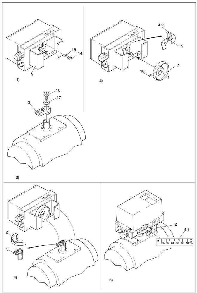
Fig. 4 Assembly sequence (rotary actuator)
