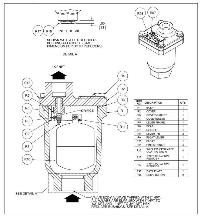
Figure 1: ARV-50A Clean Water Air Release Valve
