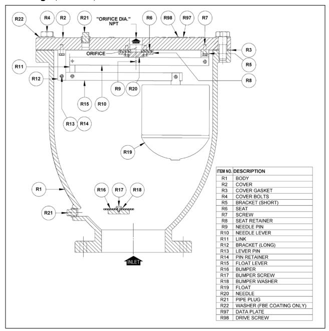
Figure 8: ARV-207 Clean Water Air Release Valve
