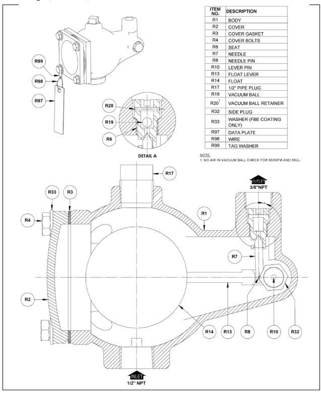
Figure 2: ARV-55 Clean Water Air Release Valve
