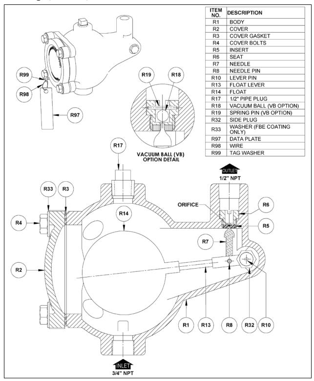
Figure 3: ARV-65 Clean Water Air Release Valve
