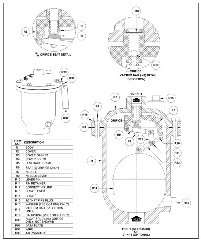
Figure 5: ARV-200A Clean Water Air Release Valve
