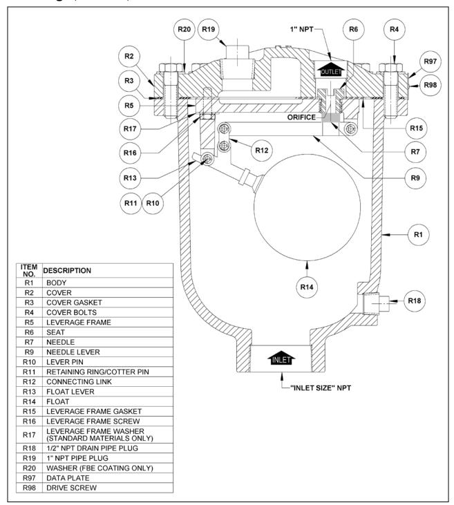
Figure 4: ARV-200 Clean Water Air Release Valve
