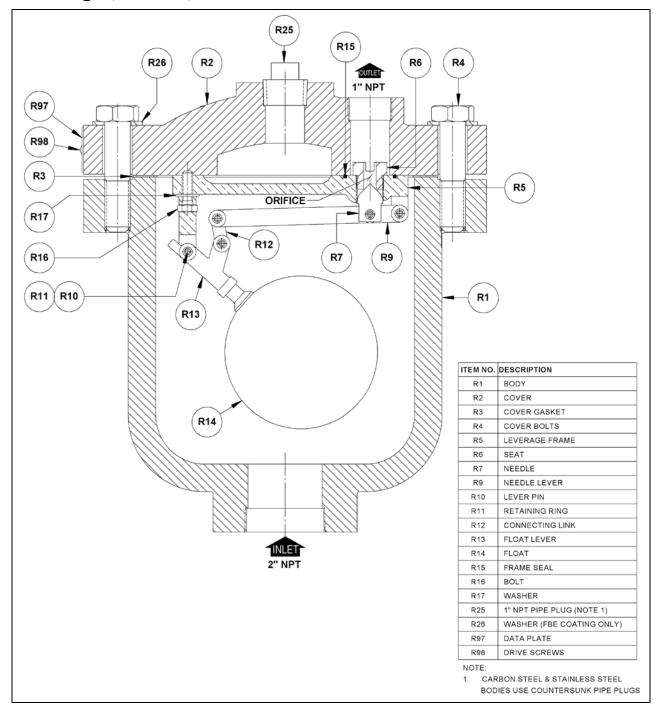
Figure 7: ARV-206 Clean Water Air Release Valve
