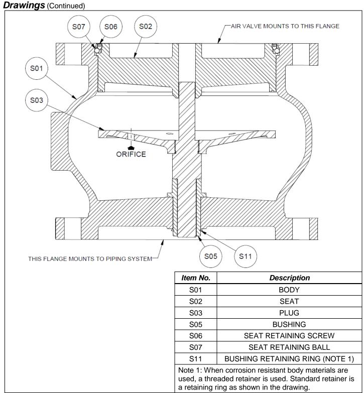
Figure 3: CSV-1600A Surge Check Valve Sizes 3-18" (80-450mm)
