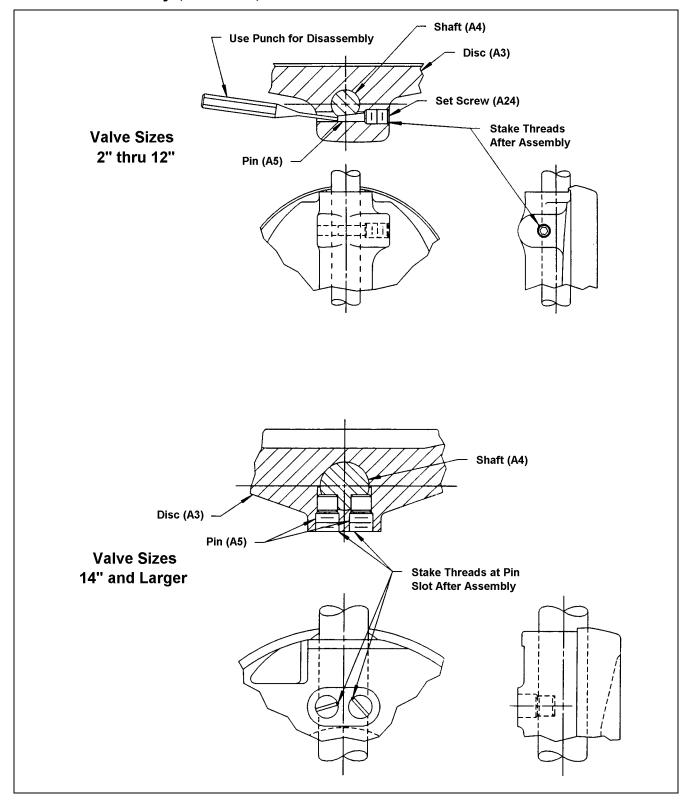
Figure 4 - Disc Pin Assembly
