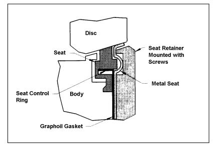
Figure 3 — (FB) Fyre-Block Seat Options (RTS2 and TTS2)
