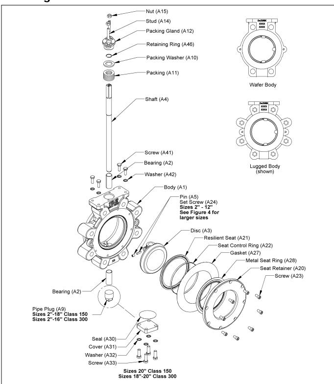
Figure 1 – Component Identification
