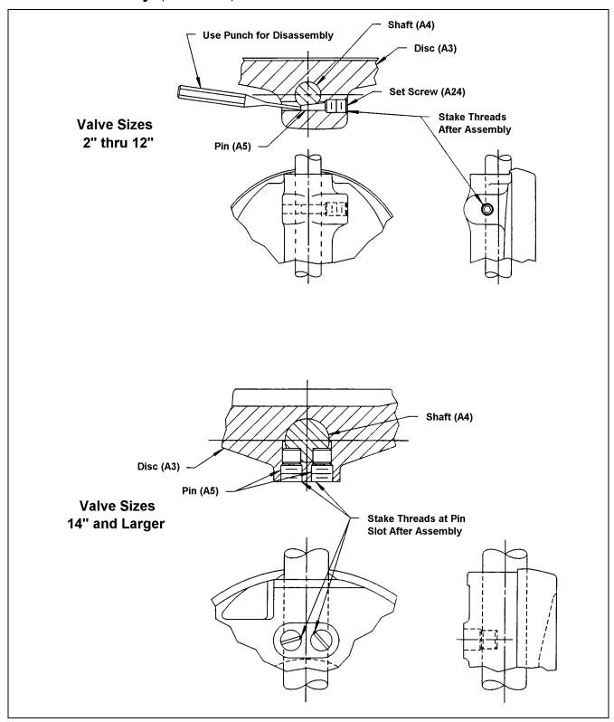
Figure 14 - Disc Pin Assembly
