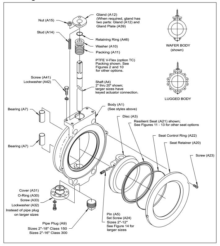
Figure 1 – Component Identification
