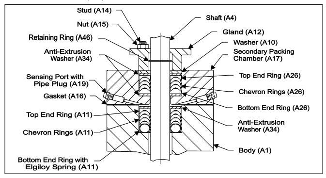
Figure 4 – Packing Option (TMD)
