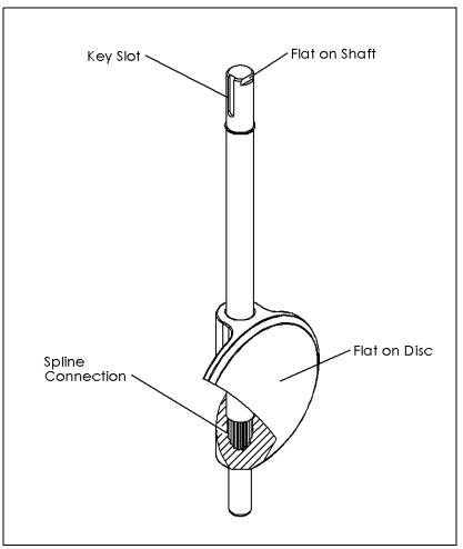
Figure 3—Disc/Shaft Alignment
