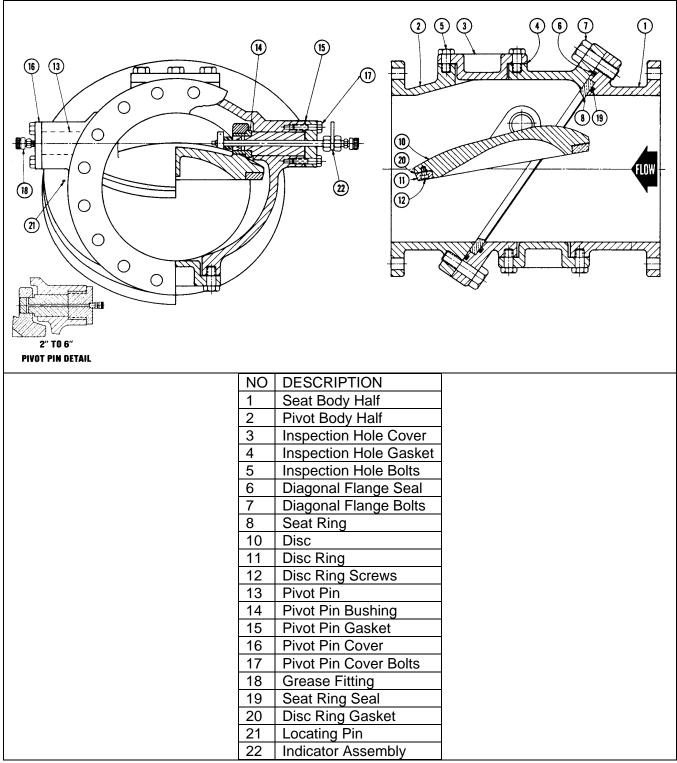
Figure 6: CSD-800 Slanting Disc Check Valve
