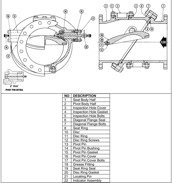
Figure 6: CSD-800 Slanting Disc Check Valve
