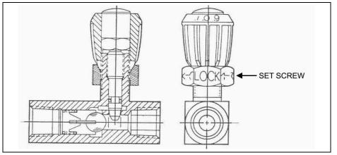
Figure 3: Flow Control Valve
