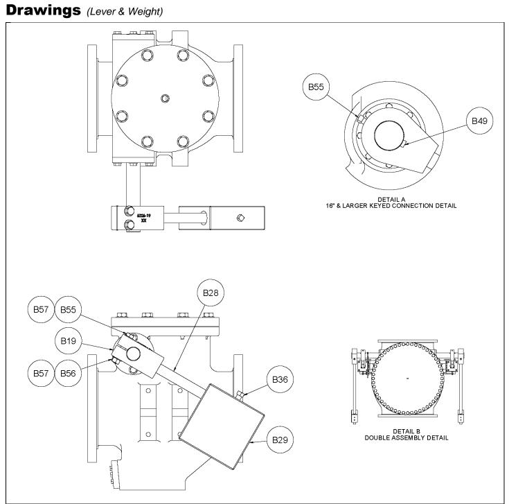
Figure 3 - CVS-6000/6000A-LW and -CLW Swing Check Valve with Lever and Weight
