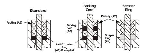
Figure 3—Packing Ring Detail
