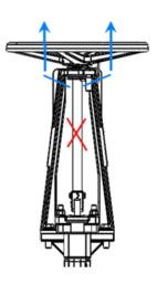
Figure 6- Knife Gate Valve with Handwheel or Chainwheel Actuator, Vertical Lifting
