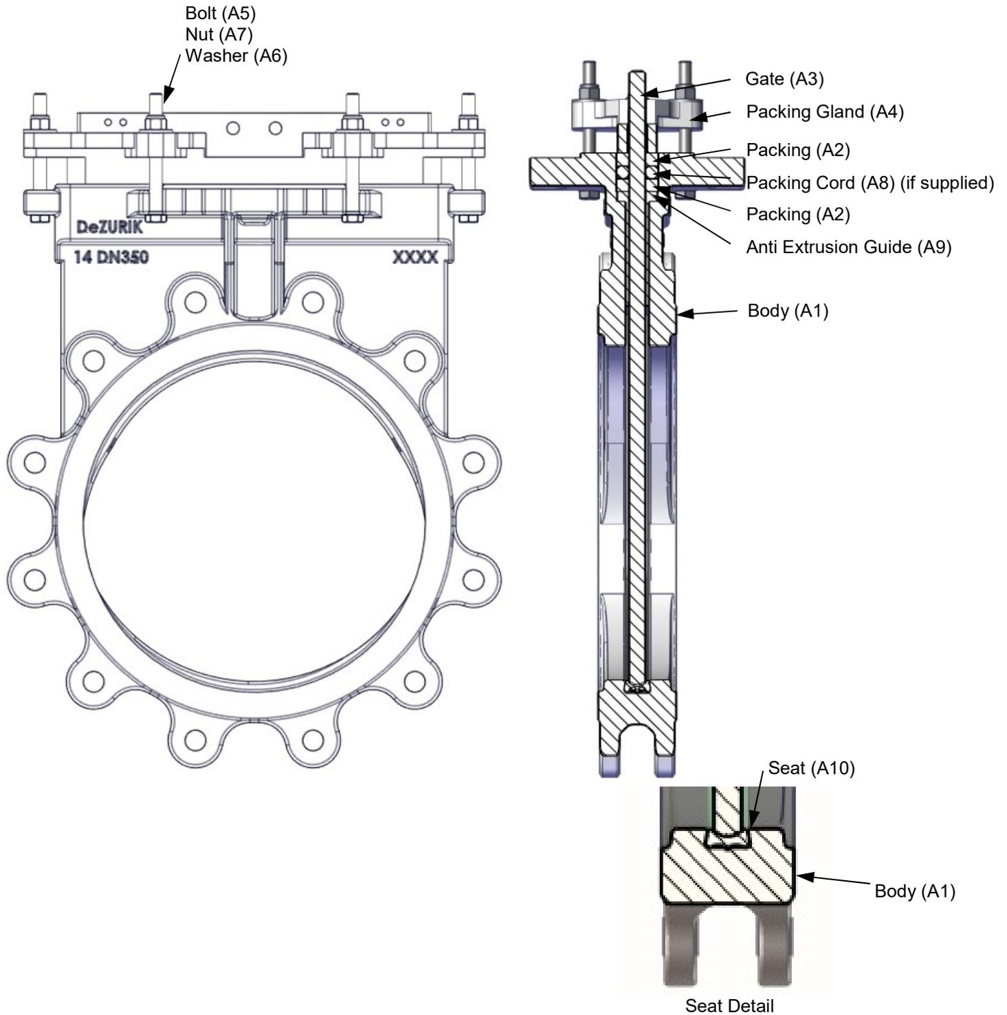
**Figure 1—Component Identification**
