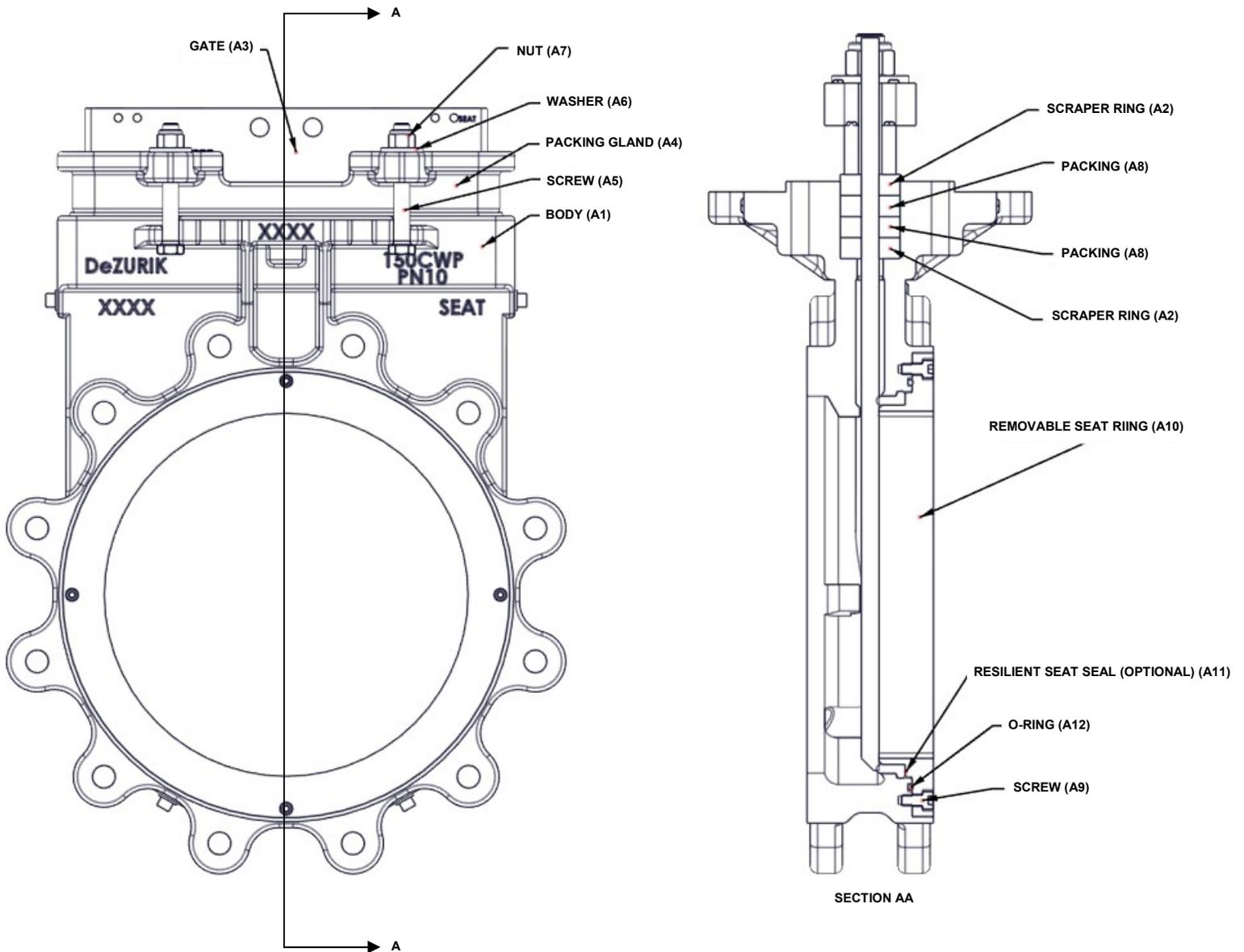
**Figure 2—Component Identification**
