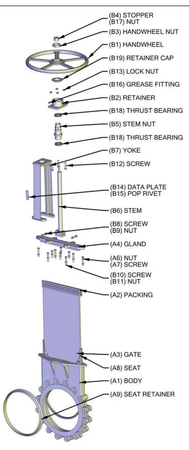
**Figure 1: Component Identification**
