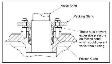
Figure 5—Friction Cone Adjustment
