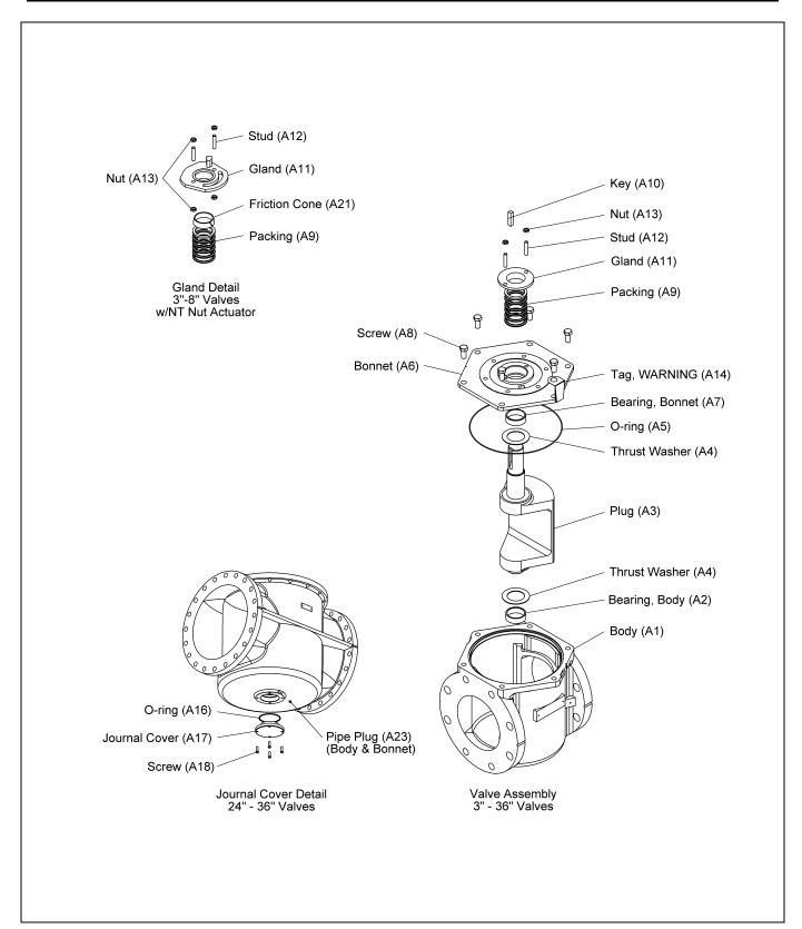
Figure 3—Parts Identification
