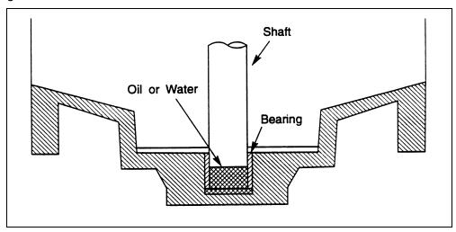
Figure 3—Hydraulically Removing the Lower Bearing
