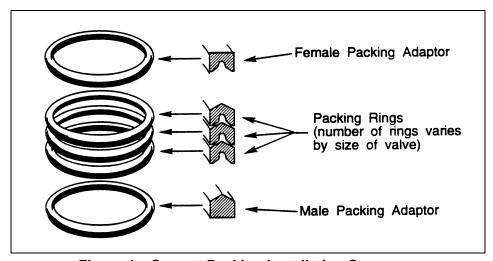
Figure 1—Correct Packing Installation Sequence
