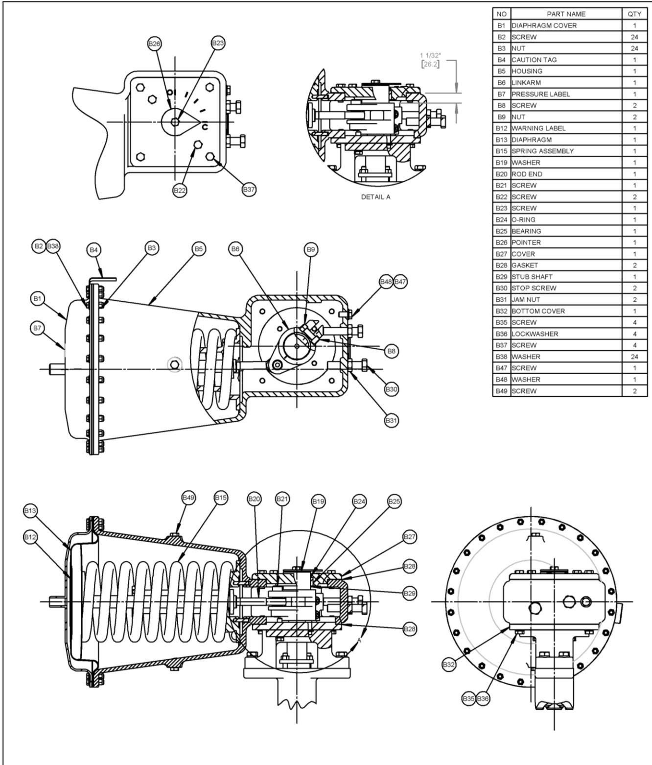
**Figure 1 - Parts Identification**
