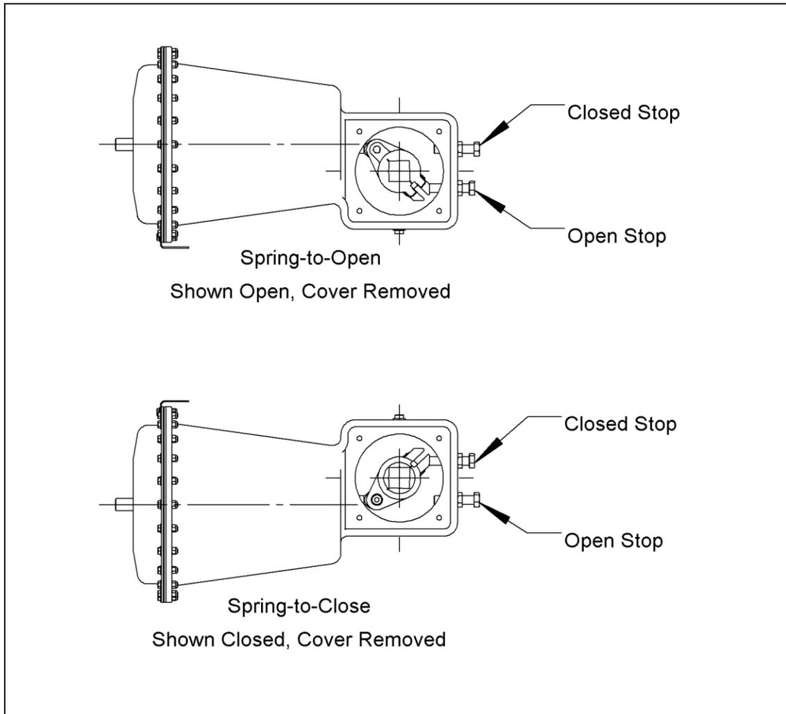
**Figure 2 - Open and Closed Position Stops**
